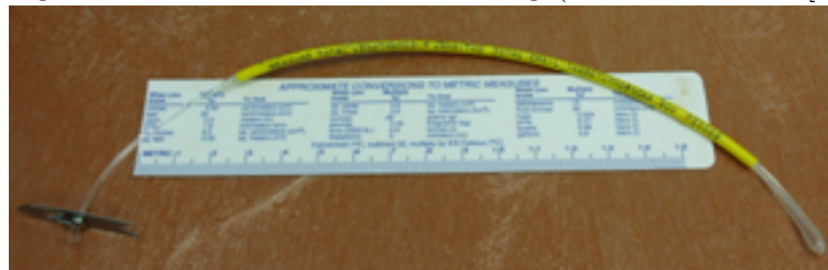
Figure 2: Detail of the newer M-tag (Source: NOAA [2])
